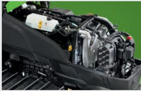
↑ Compact and efficient. FARMotion engines with optimised unitary displacement for power and efficiency, Visco fan and PowerCore air filter.
