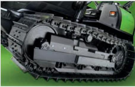
↑ Innovative undercarriage with six track rollers for superlative stability and traction.
