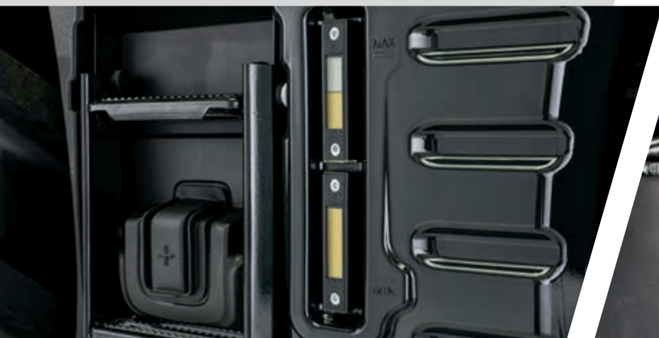
> Quick jump port and oil level glass.
