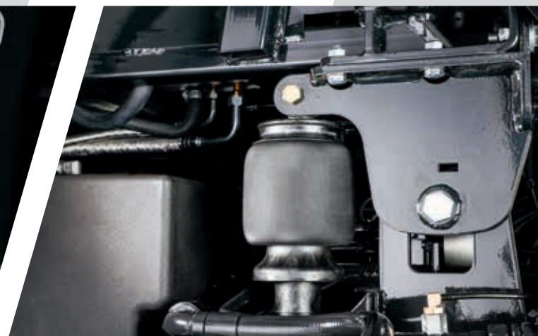
> Pneumatic cab suspension for a smoother ride.
