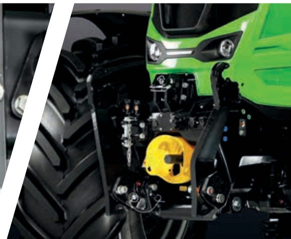
> 5450 kg lifting capacity and DualSpeed front PTO.
