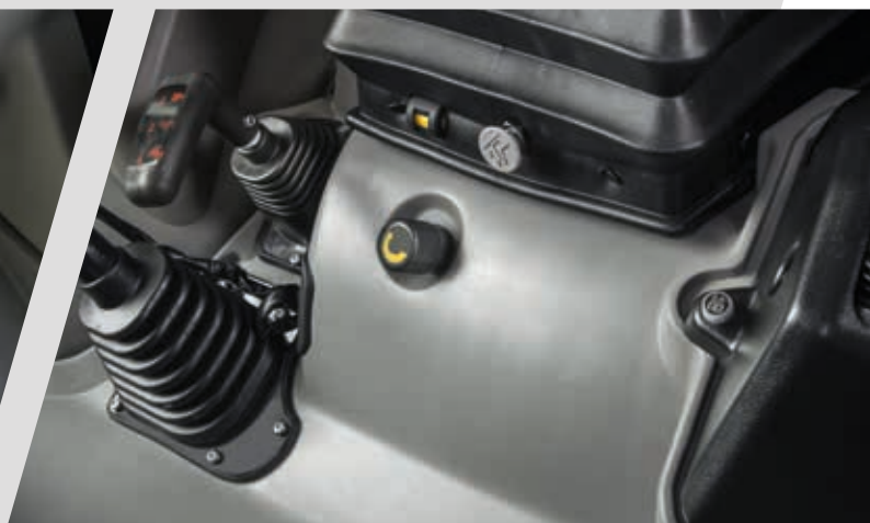
> Debietregelaar in cabine.
