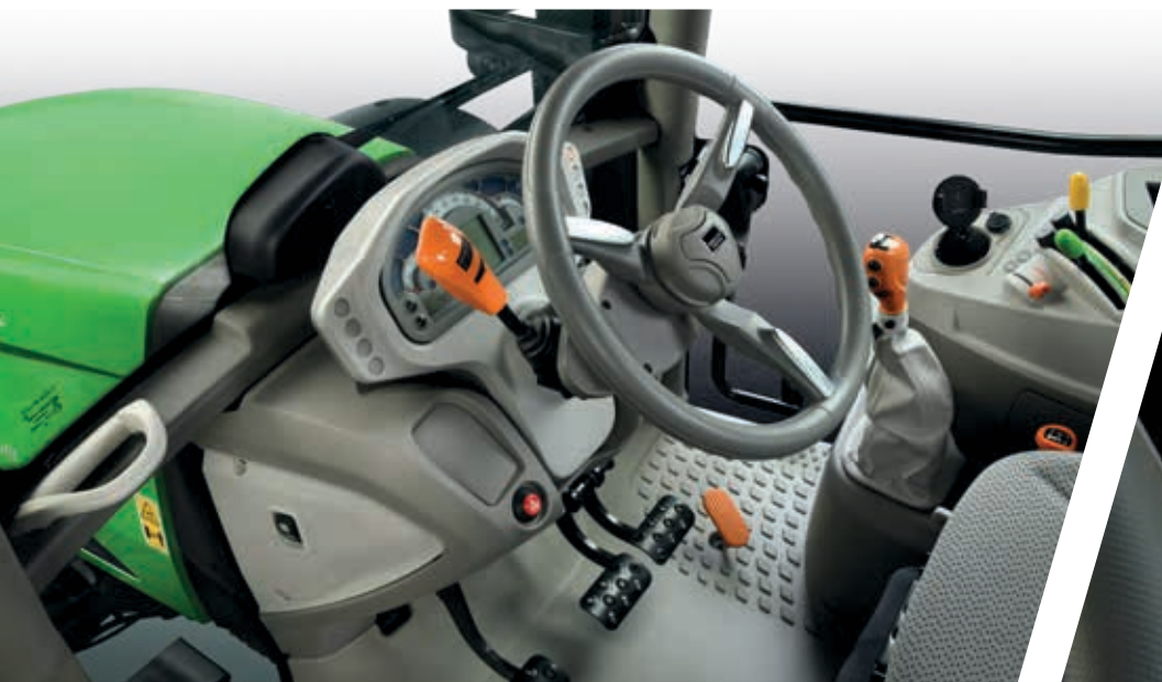
> PowerShuttle with SenseClutch 5-levels adjustment and Stop&Go function.
