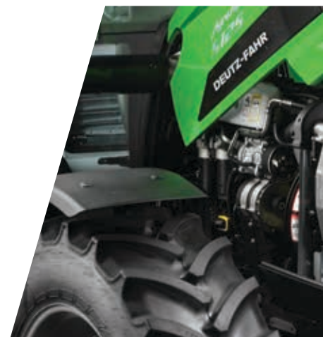
> FARMotion engine with power ratings from 75 to 126 HP.
