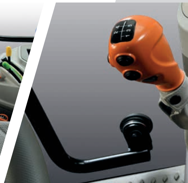
> Ergonomic gear lever with Powershift transmission controls and ComfortClutch.
