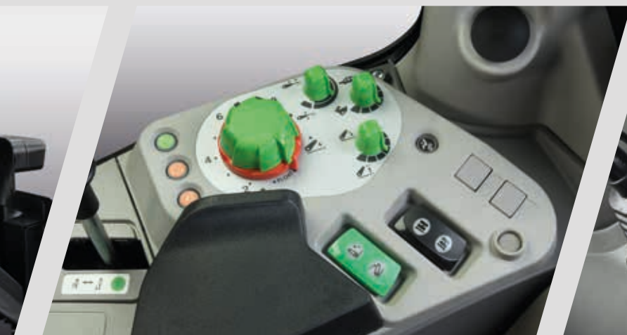
> Precise draft and position control thanks to electronic rear lift.
