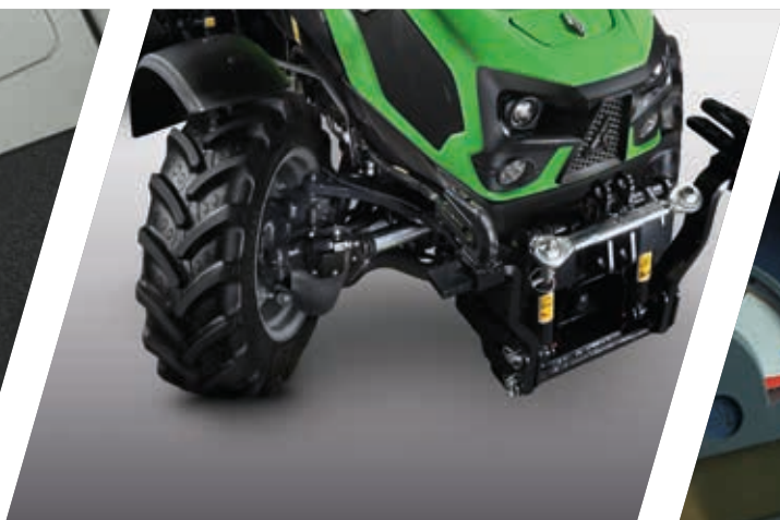
> High steering angle thanks to independent front axle suspension.
