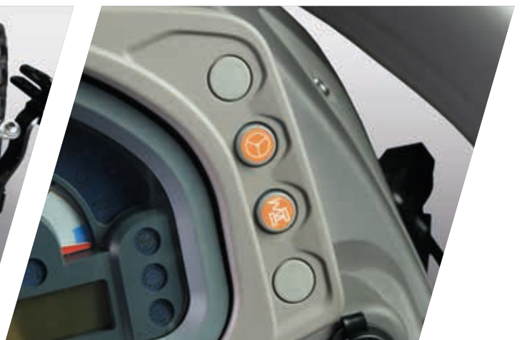
> SDD function halves the number of steering wheel turning required for lock-to-lock steering.
