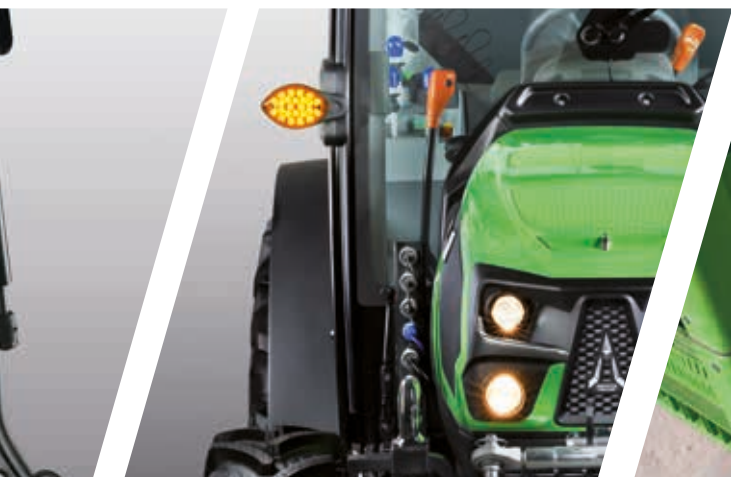
> LED position and direction lights.
