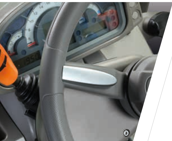
> PowerShuttle with SenseClutch 5-levels adjustment.
