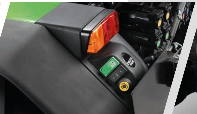
> External pushbuttons for the rear lift, rear PTO, and side stabilizers simplify coupling maneuvers.
