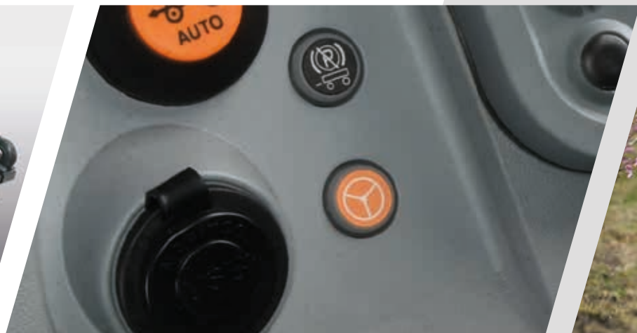
> SDD function halves the number of steering wheel turns required for lock-to-lock steering.
