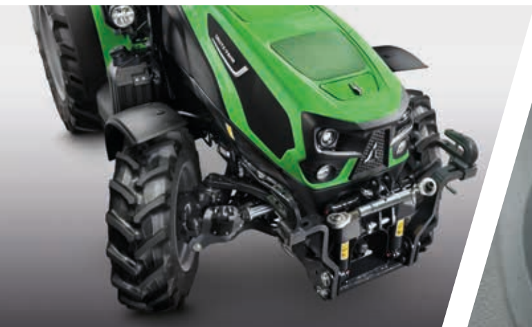
> Electronically controlled independent front axle suspension for better comfort and traction.
