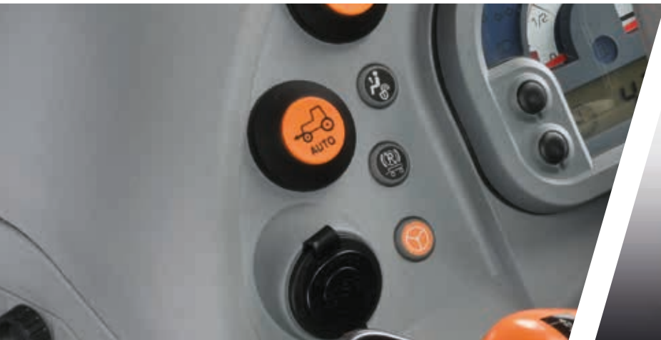
> Auto 4WD function automatically engage and disengage 4WD according to steering angle.
