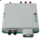
Device required to receive an RTK NTRIP correction signal (centimeter level precision guidance)
